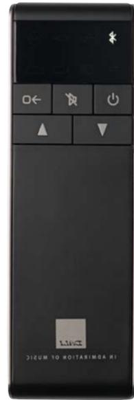
The Sound Hub **remote control** connects via Bluetooth, so the Sound Hub can be hidden out of sight if desired
